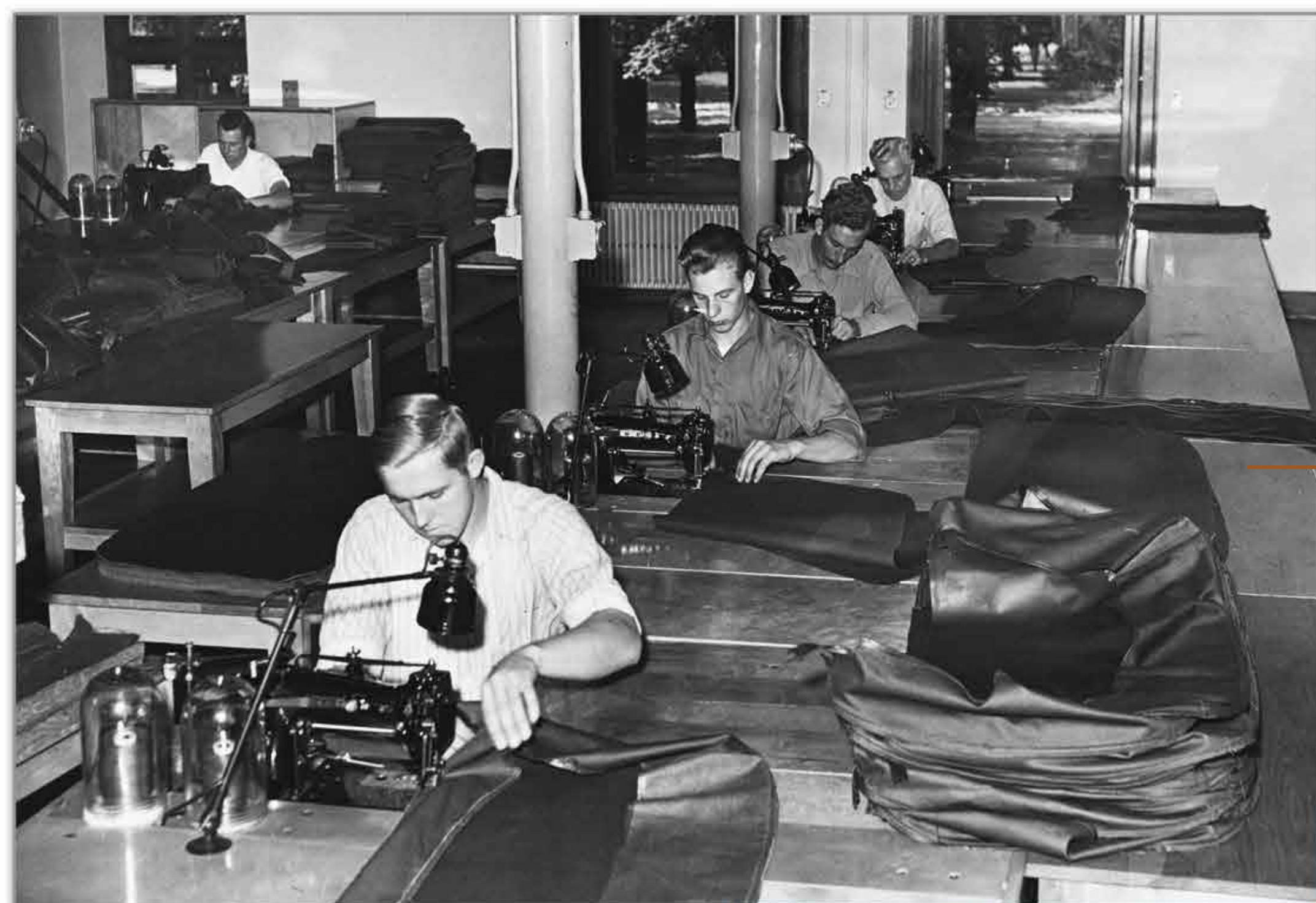
Workers assemble vehicle seat cushions within the former school building, early 1940s. From the collections of The Henry Ford.
